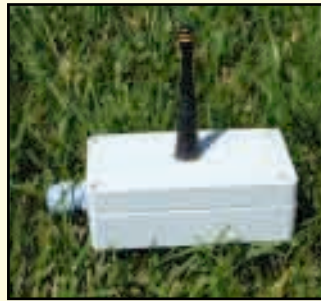
Satellite Pedestal Repeater
