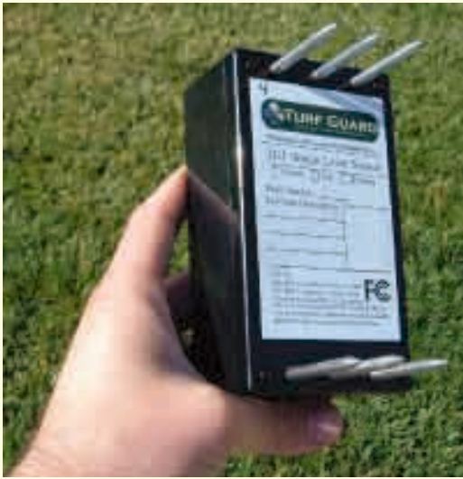
TG1 Wireless Moisture, Temperature and Salt Level Sensor
